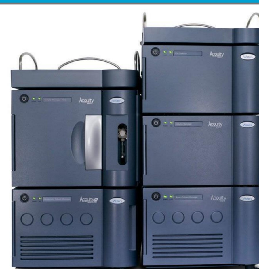
Figure 2: UPLC-UV-MS(QDA) from WATERS that is used during the project
